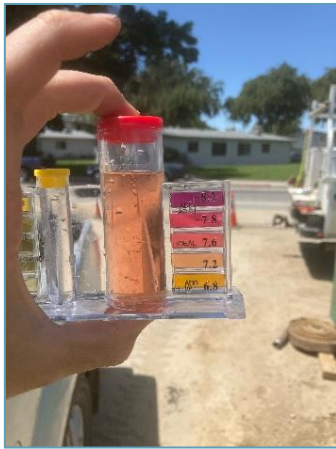
Trench dewatering monitoring prior to discharge into City's sewer system
