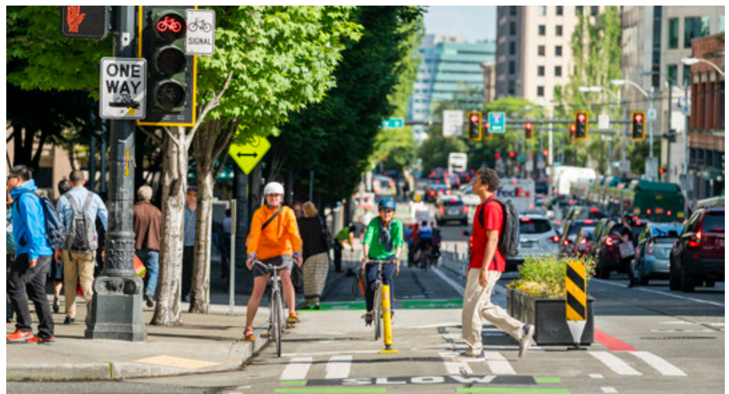
Figure 3.38 An example of a street retrofitted with a protected bikeway using low-cost techniques. This can be an approach to consider for G and H Streets.
